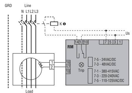
① The coil connection can vary depending on the connected type of device (contactor, breaker with shunt trip release or breaker with undervoltage trip release).
