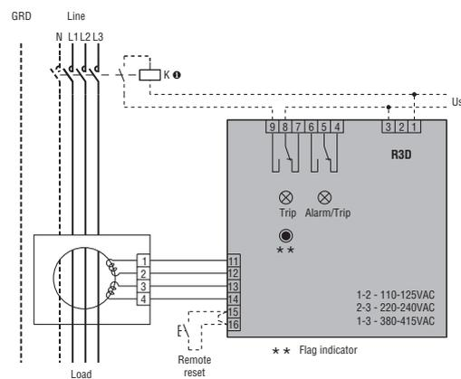
① The coil connection can vary depending on the connected type of device (contactor, breaker with shunt trip release or breaker with undervoltage trip release).
