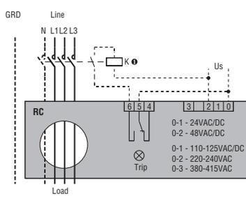
① The coil connection can vary depending on the connected type of device (contactor, breaker with shunt trip release or breaker with undervoltage trip release).
