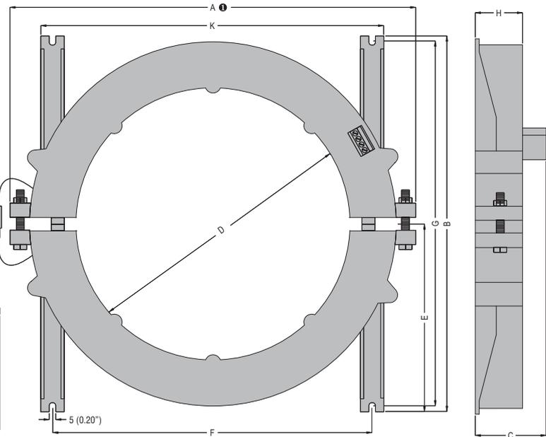
● With screws, for RTA210 split-core type; fixed structure, without screws, for RT210 type.
