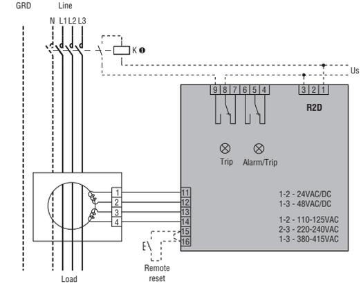
① The coil connection can vary depending on the connected type of device (contactor, breaker with shunt trip release or breaker with undervoltage trip release).
